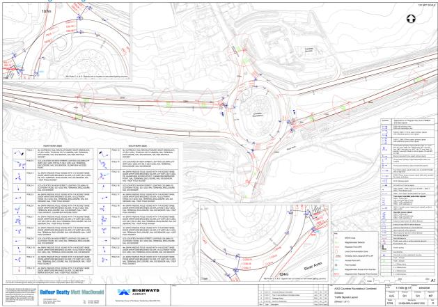
The traffic signal design for the roundabout
